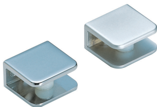
Glass Standoff - 2880 Glass Thickness: 1/4"~ 3/8" (6~10 mm) Material: Zinc Alloy or 304 Stainless Steel
